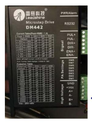
If the numbers provided do not work check your Y Axis controller to see what the Pulse/Revs are for the given DIP Switch positions. (see photo)
